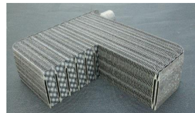
Figure 3: Heat Exchanger designed and built at CIMP-3D at Penn State using the powder bed fusion process and sliced to show internal structure.
