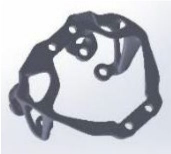
Topology optimized Motor Bracket for Lunar Lion Satellite Module
