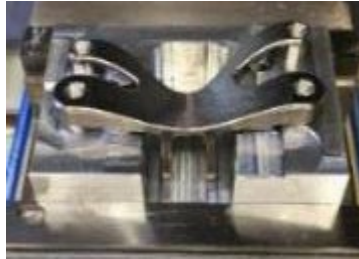
2 nd Op Machining Completed
