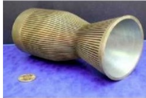
Rocket Thrust Chamber Printed from Functionally Graded Metal
