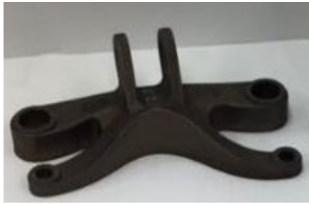
Laser Powder Bed Fusion Build L-PBF Part with Supports after Separation from the Build Plate
