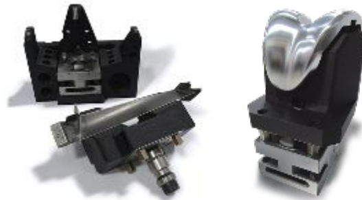
Prototype PAAW Fixtures Printed from Carbon Fiber Reinforced Nylon
