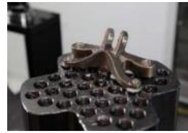
Bracket Support Bonded to PAAW Fixture for 1 st Op
