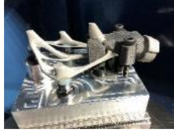
Hybrid PAAW for AM Application (Renishaw)
