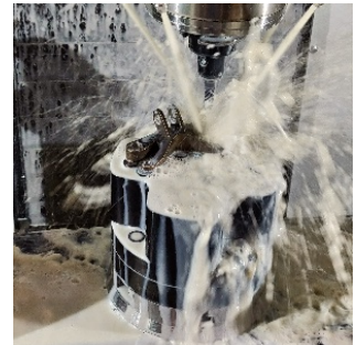
Five Axis Machining of GE Aviation Bracket using Modular PAAW Fixture
